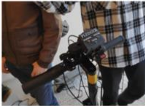
Testing of VRU gadget, tuning LEDs and buzzer
