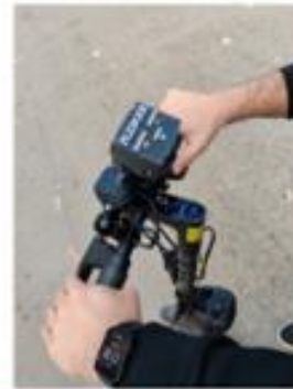
Testing of VRU gadget, tuning LEDs and buzzer
