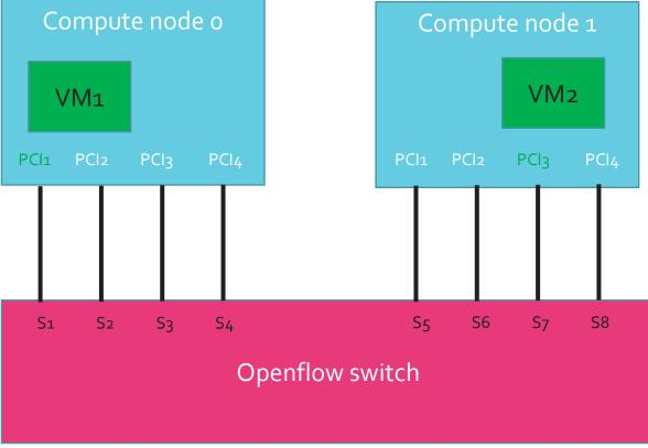
VM2 will be e.g. deployed in compute node 1 and will consume interface identified by PCI address PCI3 and MAC MACY
