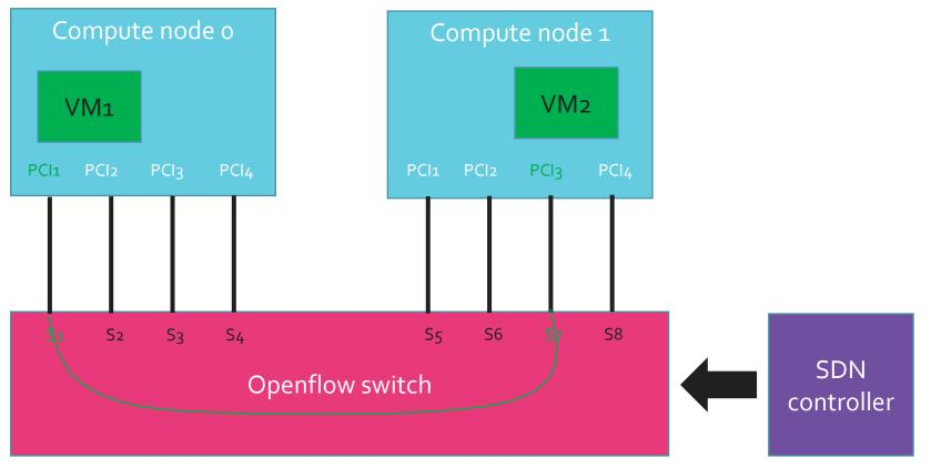
Example of rules for E-LINE and PCI passthrough interfaces: IN: Port S1  $\rightarrow$  OUT: Port S7 IN: Port S7  $\rightarrow$  OUT: Port S1
