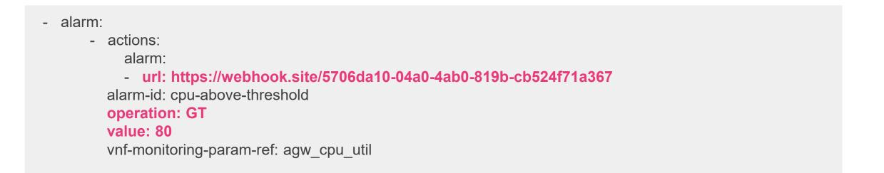
Alarms based on metric thresholds can be sent to webhooks The alarm descriptor is also part of a VNFD. Like the example shows, it mainly specifies:
